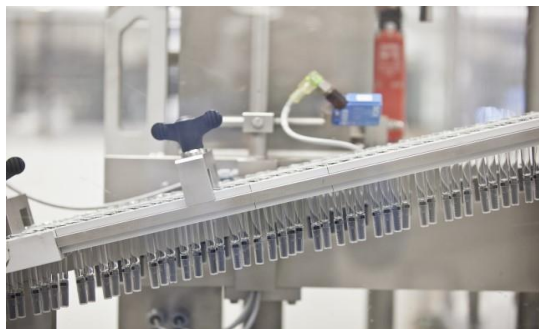
Figure 3. Automated Syringe Inspection, Labelling and Packaging Lines can process 300 units per minute.
