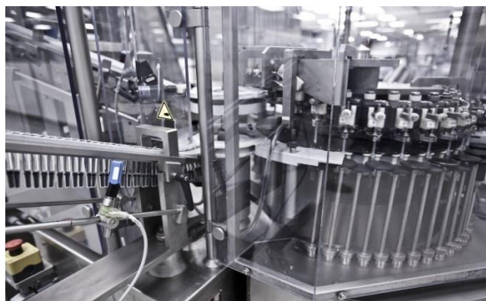
Figure 1. Automated Plunger Rod insertion in Filled PFS units.
