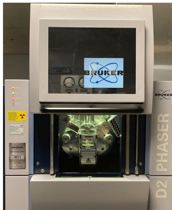
Figure 5. Bruker D2 Phaser Instrument housed in R&D of Baxter BioPharma Solutions.
