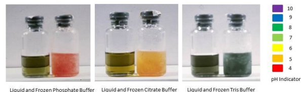
Figure 2. pH shift in between liquid and frozen states for phosphate, citrate, and Tris buffers.
