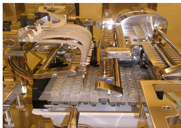
Figure 6. View of Filling Syringes Followed by Stopper Placement Using an Insertion Tube.
