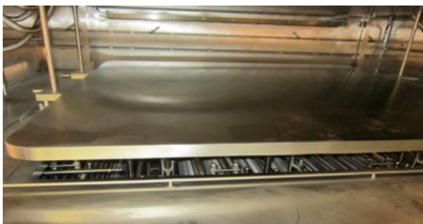
Figure 3. Lyophilizer Equipped with an Adjustable Platform Between the Product Chamber and the Condenser.
